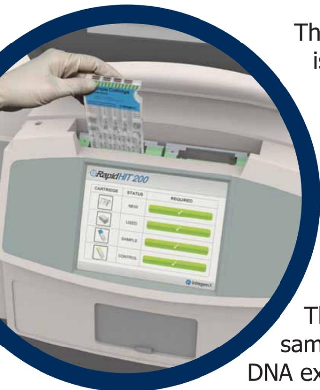
The forensic community is continually striving to improve the analysis of DNA, particularly with the development of more rapid and efficient processing techniques. The first commercially available solution is the **IntegenX RapidHIT®200 instrument**. The instrument integrates sample handling steps through DNA extraction, normalisation, amplification, separation and detection.
